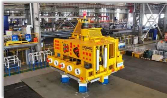
Key R&D products: 2000m class ultra-deepwater X-mas tree
