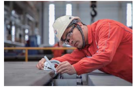
The construction personnel measured the groove accuracy of the processed plate
