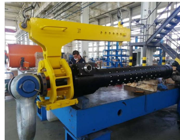
▲ Emergency Recovery Device for Subsea Pipeline
