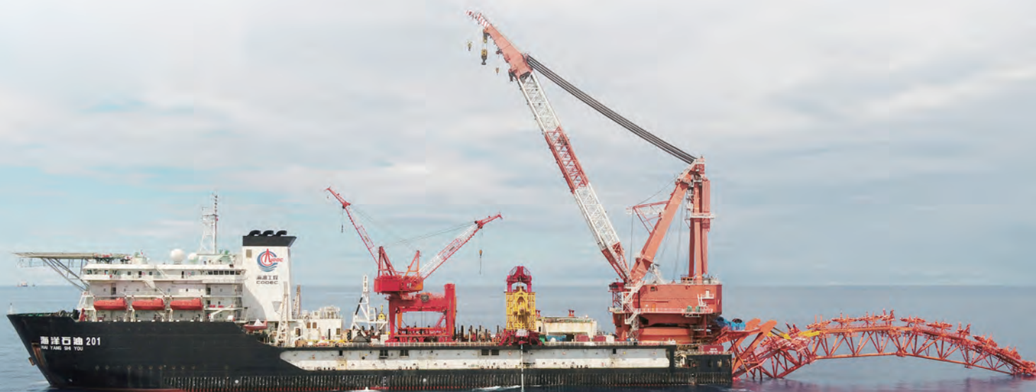
SCR S-lay installation in 1500 m ultra-deep water
